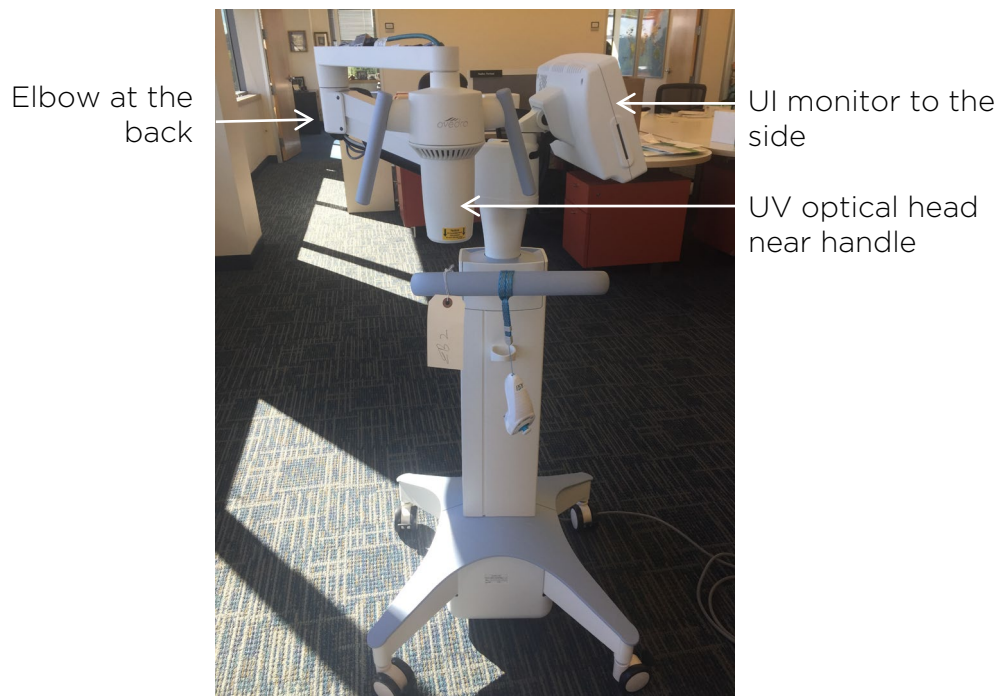
Figure 4-2. Moving System Configuration
