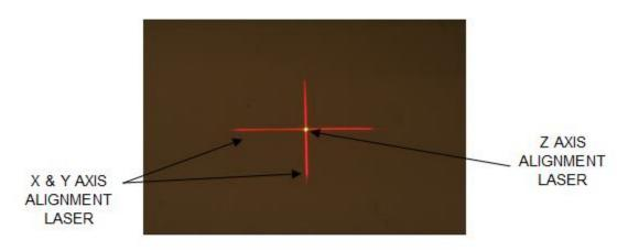
Figure 3-21. Red Crosshairs X & Y Axes, Green Dot Z Axis Alignment
