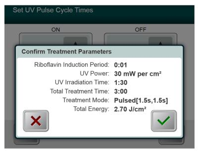
Figure 3-10. Confirm Pulsed Treatment Parameters Screen
