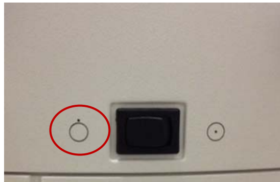
Figure 3-32. Power Off Position
