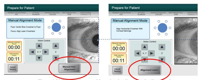
Figure 4-20 Toggling between Manual Axis Alignment & Alignment lasers
