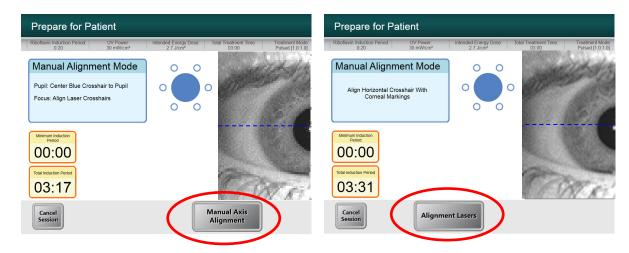
Figure 5-25. Toggling between Manual Axis Alignment & Alignment Lasers
