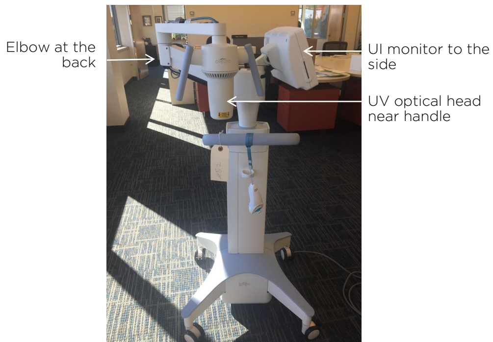
Figure 4-8. Moving System Configuration
