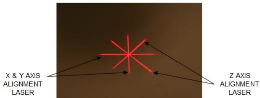
Figure 3-23. Alignment of Red Crosshairs – X & Y Axes and Z Axis
